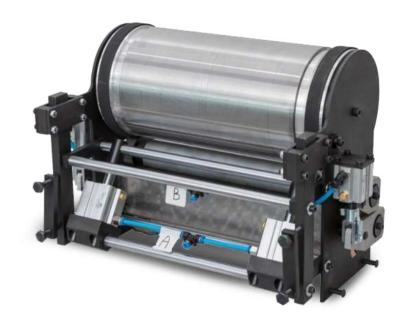
Inline Printers are equipped in blown film extruders in order to print single colour prints easily and in low cost without needs of extra roll to roll flexo printing machine.
